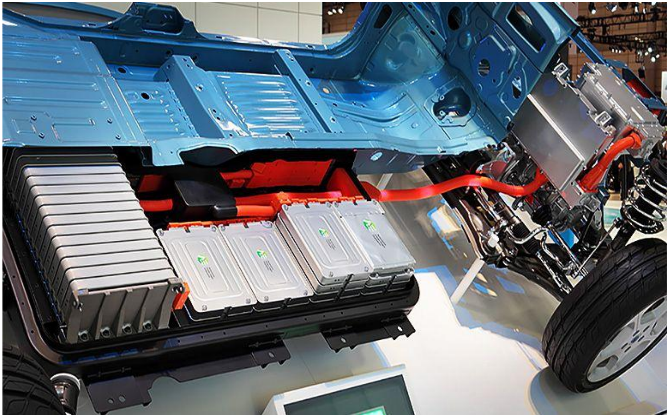
Lithium-ion battery pack in a Nissan Leaf.
