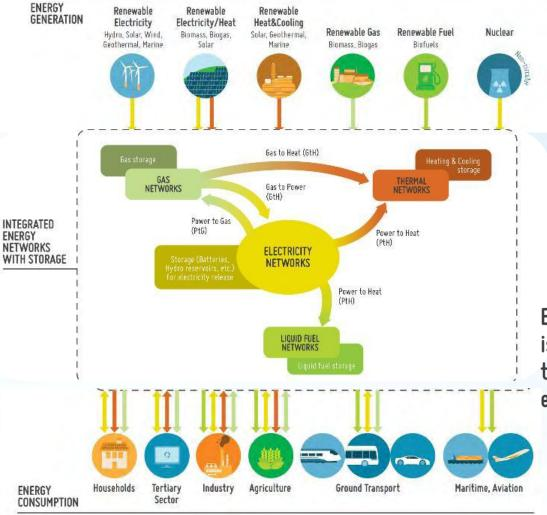
Electricity network is the backbone of the integrated energy system
